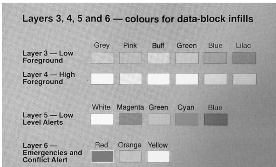
Here, the degree of intensity of color corresponds to the level of alert (collision potential) involved with the corresponding aircraft. The red, orange, and yellow labels are the most intense, and correspond to imminent collision. Linda Reynolds, the project's designer explains her group's thinking behind this intensity range.
